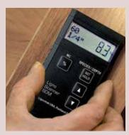
The plywood can be measured from the backside on the  $\frac{1}{4}$ -inch setting. The meter also measures vertical, horizontal and strand bamboo on the  $\frac{1}{4}$ -inch depth setting.
