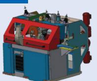
SideMaster provides side matching for sawnface engineered wood flooring and plan-tozero systems. The HSSM Splitter produces sawn veneer faces up to 8 inches wide
