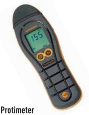
The Protimeter Surveymaster, a dualfunction moisture meter, is designed to provide a rapid assessment of building moisture with both pin and noninvasive measurement capabilities, the company says, adding that it has rugged construction and a large backlit display. It can be used in new construction, refurbishing, building surveys, fire and flood restoration, concrete and wood floor moisture measurement.
